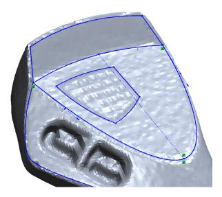
2D and 3D sketches can occur directly on the scanned mesh.
