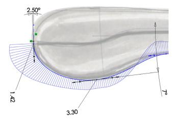
Sketch splines are displayed with handle control constraints, so you can dimension both the tangent length and angle vector of the spline point.
