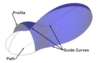
Sweeping with multiple paths, guide curves can easily produce complex shapes.
