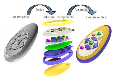
Creating individual components from the master form multiple bodies are derived to separate parts and then reassembled into a main assembly. When the master model is altered, all changes are propagated into the final main assembly.
