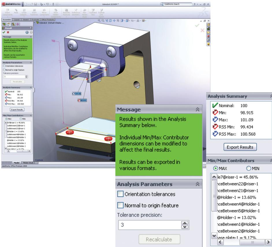
SolidWorks software provides a range of DFM tools for addressing fit and function issues, such as the TolAnalyst shown here, which automates tolerance stackup analysis. Using other SolidWorks software DFM tools to make sure that your parts will fit together for assembly, you can:
